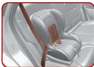
Securing a child restraint system with a lap/shoulder belt [3].
