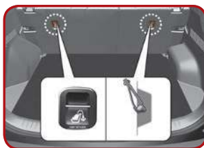
Securing a child restraint system with "Top-tether anchorage" system*. Refer to Owner's Manual [3].
