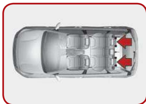
Securing a child restraint system with "ISOFIX" system. Refer to Owner's Manual [3].
